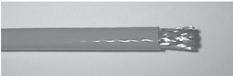
1. Remove 15 mm of the outer sheath.
