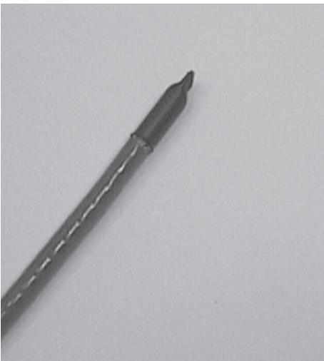
3. The crimp tube is crimped down, whereafter the outer 5 mm is squeezed with a pliers.
