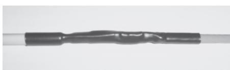
15. Make sure that the glue is running out from both ends of the crimp tube.
