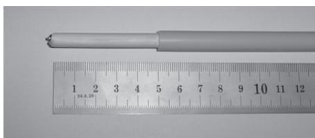
4. Remove 50 mm of the outer sheath.
