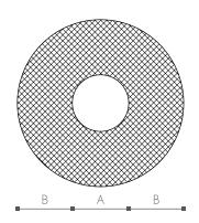
INSUL-TUBE® HI-TEMP is made of temperature resistant EPDM and maintains its flexibility even at temperatures of 150 °C (continuous operation) or 175 °C (peak usage) while maintaining the integrity of its technical properties.
