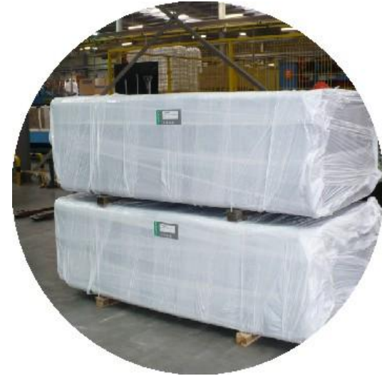
Longer pipes on pallets protected with plastic stretch
