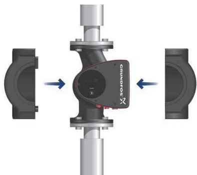
Fig. 18 Fitting the insulating shells to a MAGNA1 pump
