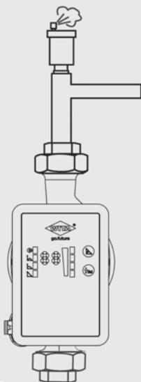
Fill and vent the system correctly. To vent the pump, loosen the indicated screw by turning it anti-clockwise. Caution! Hot water may escape here, depending on the system's operating state. Afterwards, re-tighten the screw and start the venting programme (see section 7.6 on page 37).
